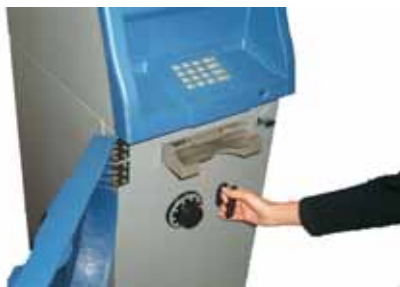
Fig. B-3 Replenishing the Cash Cassette
